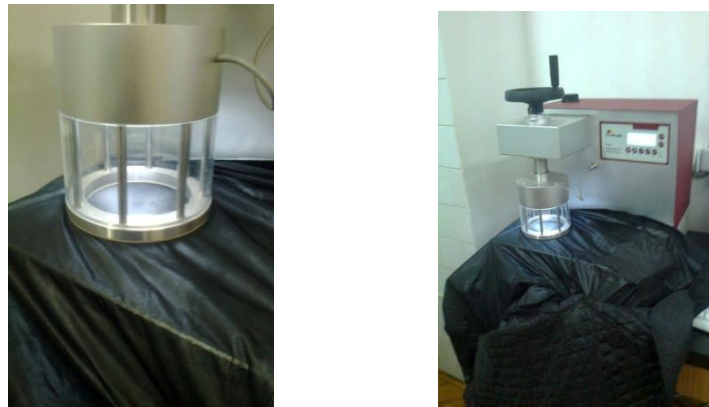
Figure 3. Determination of resistance to water penetration on the hydrostatic pressure tester according to the ISO 811 standard [6]
