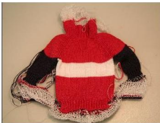
Figure 7. Seamless product – integral knitting
