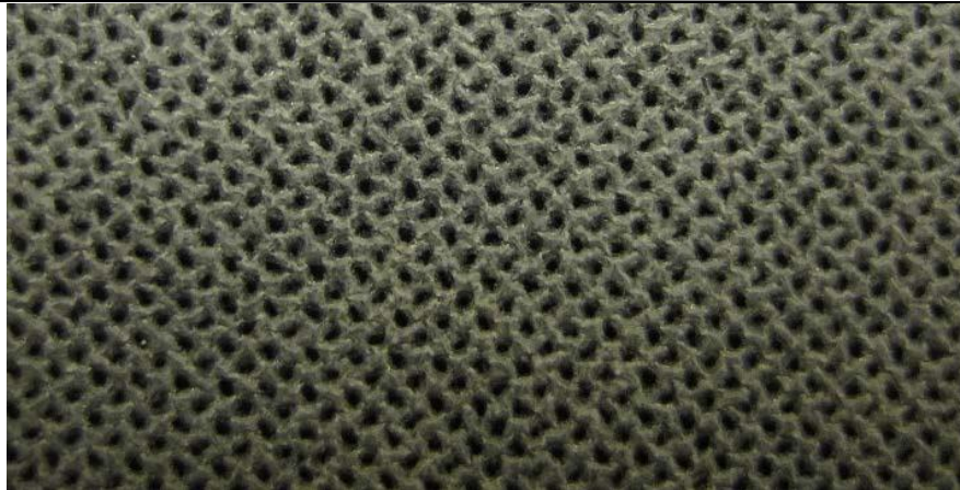
Figure 8. Climate membrane after 10 washes at a temperature of 40 ° C
