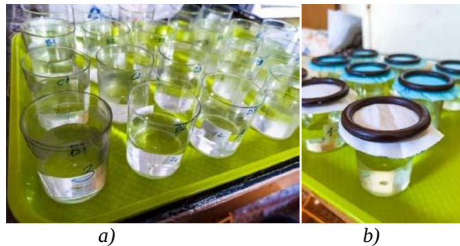
Figure 2. Water vapour permeability measurement: a) sample cup, b) open cup
